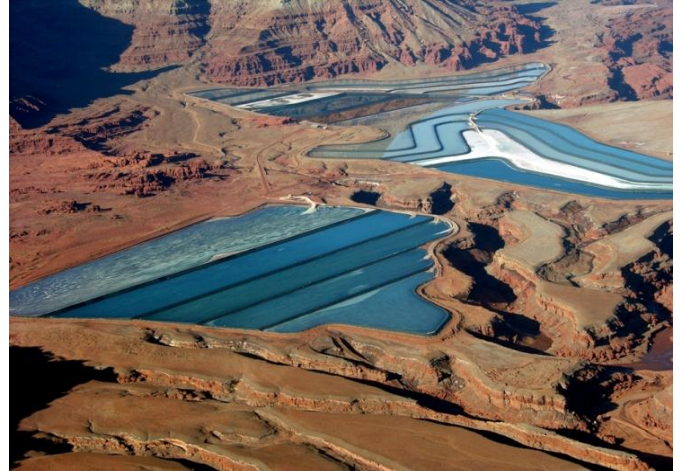
A view of the solar evaporation ponds at the Moab, Utah Intrepid Potash facilities, operating since 1972
